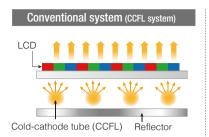
The CCFL system requires the installation of multiple tubes that illuminate in the same way as fluorescent lamps behind the LCD panel. Thus, the display unit becomes thick
