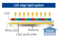
The edge light system requires a small number of LED units because the lights are installed only on the edges of the LCD panel. This saves energy. The display unit can also be made thin and light.
